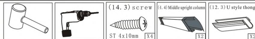
Set the middle upright column(4.4)to connect with fixed glass other sides.Fix middle upright column by screw ST4\*10mm(14.3).
