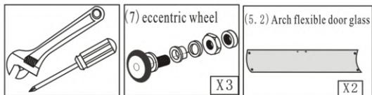
Set eccentric wheel(7)into arch flexible door glass topmost holes.Fix the wheel and hang the door up into rails, and fit the wheel into bottom holes then,and adjust the wheel by spanner,to make the door go and back smoothly.
