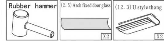
6. ) Fit the fixed glass into the frame, after fitting the rubber seal into glass one side, and then knock the glass carefully by hammer.
