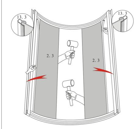
Installing fixed glass.take off aluminum alloy water barthen install water dar after installing fixed glass and aluminum panel
